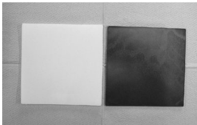
Figure 7 Photographs of composite plate samples (150 mm \times 150 mm \times 3 mm): 100 wt % MPE (on the left) and 80 wt % MPE and 20 wt % Clay (on the right).
